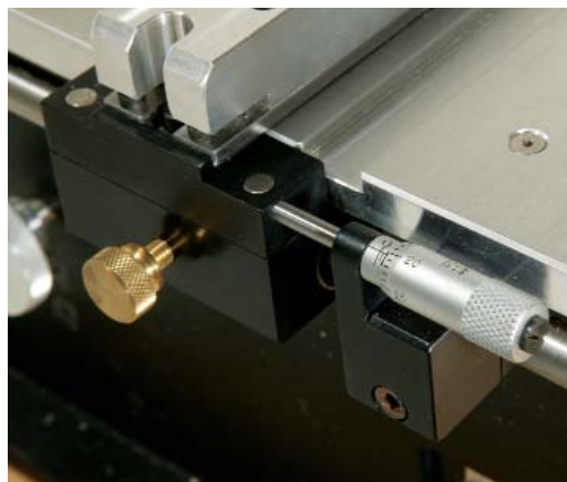
This Starrett micrometer head can be positioned to provide precise control of the fence to one one-thousandth of an inch.
