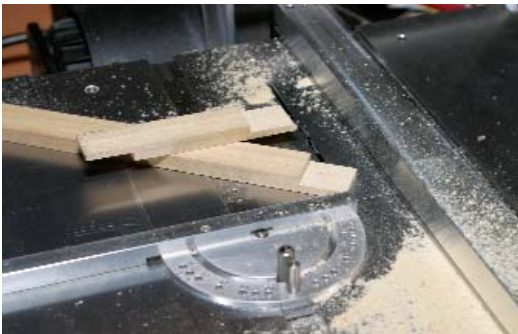
I milled these pieces of poplar and cut these precise test lap joints in just a few moments while making a vacuum forming frame.
